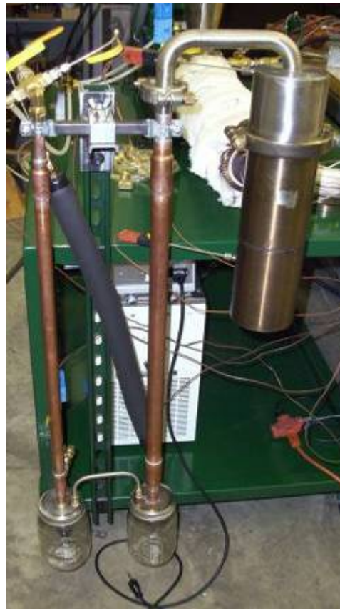
Condenser and collection vessels
